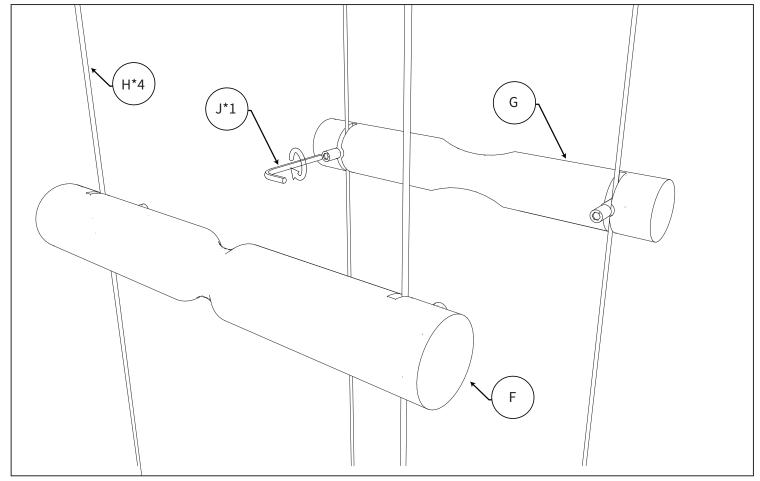
Note: Solid structural backing is required - 3/4" plywood is recommended. I\*8 A\*8 D\*4
